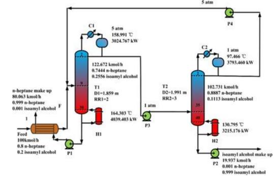
Fig. 5. The most energy-efficient process of pressure-swing distillation.
