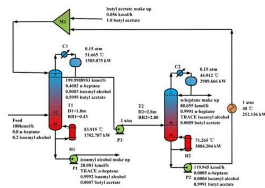
Fig. 4. The most energy-efficient process of extractive distillation
