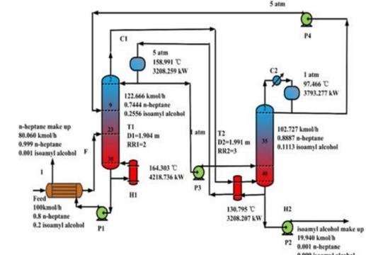
Fig. 6. The most energy-efficient process of pressure-swing distillation with full thermal integration process.
