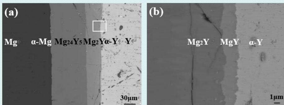
**Figure 1.** (a) BSE images of the Mg/Y diffusion couple interface annealing at 673 K for 170 h. (b) magnified view of Y side at the interface. (c) Y solute concentration profile through the diffusion interface.
