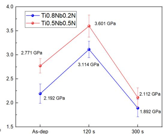
Fig. 5. Hardness of the as-deposited coating and the coatings oxidized at 500 °C for 120 and 300s.
