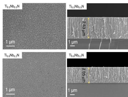
Fig. 3. Surface and cross-sectional morphologies of  $Ti_{0.5}Nb_{0.5}N$  and  $Ti_{0.8}Nb_{0.2}N$  coatings.
