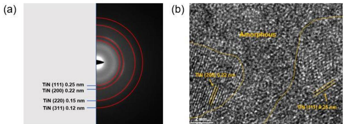
Fig. 6. (a) Fast Fourier transform (FFT) derived diffraction patterns of  $Ti_{0.5}Nb_{0.5}N$  coating oxidized at 500°C for 120 s and high-resolution (HR) TEM image
