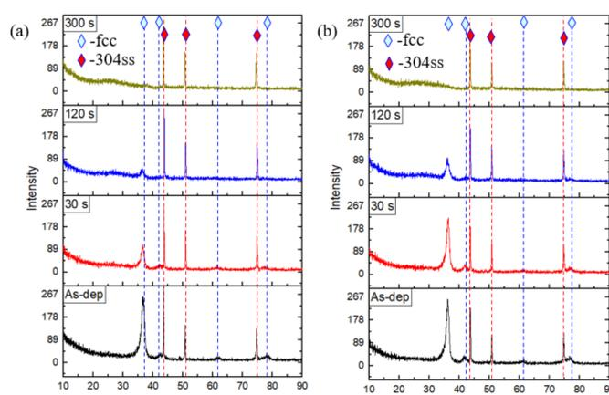
Fig. 4. XRD patterns of the coatings in the as-deposited condition and after oxidation at 500 °C for 30, 120 and 300s: (a)  $Ti_{0.5}Nb_{0.5}N$  and (b)  $Ti_{0.8}Nb_{0.2}N$ .
