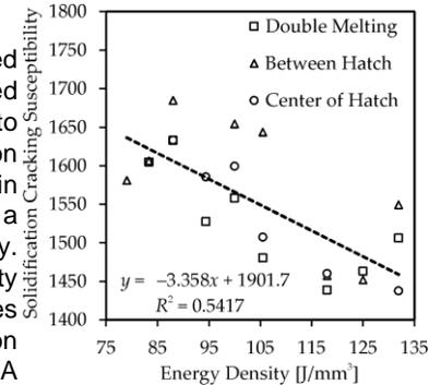
Figure 4. Solidification cracking susceptibility of stainless steel 316L as a function of energy density
