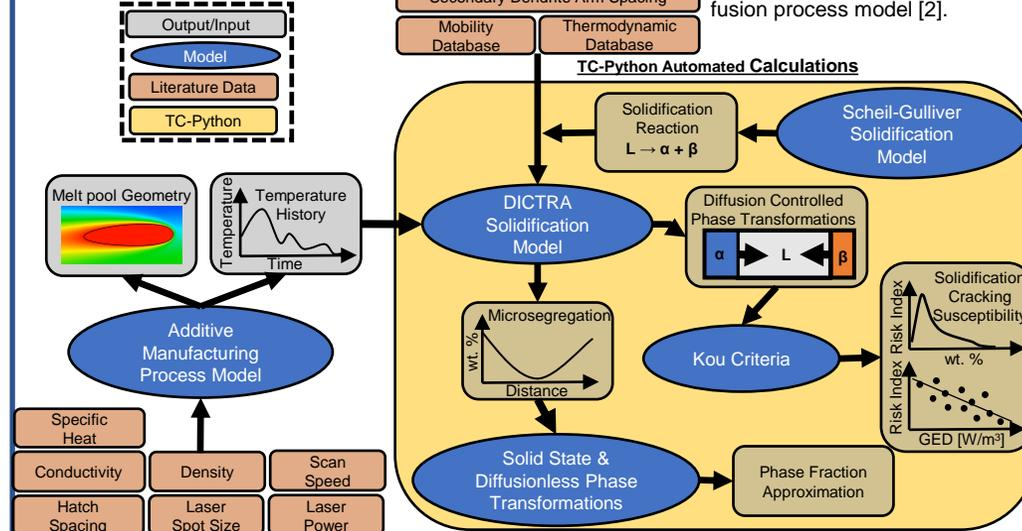
Figure 3. CALPHAD-based ICME (CALPHAD: Calculation of Phase Diagrams, ICME: Integrated Computational Materials Engineering) framework for modeling non-equilibrium solidification of additively manufactured materials. This modeling framework integrates processing and microstructure models for non-equilibrium solidification.
