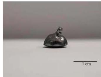
Figure 2i.: Si arc-melted sample, view: 2
